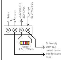
Voltage from +24V Out through resistor to Trigger Input holds power to receptacle "ON." Shunting Trigger Input to Com via Fire Alarm Panel contact closure forces power to receptacle "OFF."
