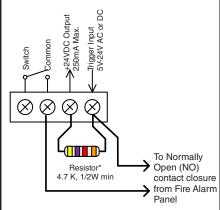
Voltage from +24V Out through resistor to Trigger Input holds power to receptacle "ON." Shunting Trigger Input to Com via Fire Alarm Panel contact closure forces power to receptacle "OFF."
