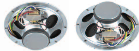
The assembly features two factory-mounted drivers with 70V transformers — one firing up to shape background noise for sound masking, one firing down for music and paging.
