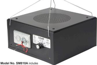
8" 15W driver with transformer, black grille, black backbox with externally accessible leads and single gang input plate, and mounting hardware (4 ft. chain with S-hooks and pre-mounted wire hangers).
