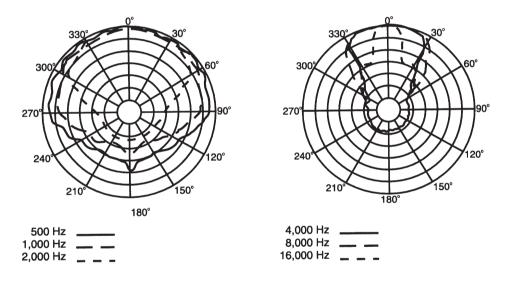
Polar Response in 1.8 ft<sup>3</sup> Sealed box 4 volt RMS of 1/3 octave Band Limited Noise in Anechoic Environment, 20 feet on Axis.
