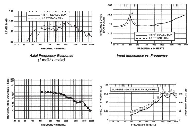
Beamwidth vs. Frequency in 1.8 ft<sup>3</sup> Sealed Box
