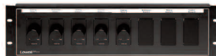
Rackmount Panel No. D8P-ID-3: mounts up to 8 Decora style 1-gang devices. Photo shows LVC Series Decora controls and blank plates for unused positions. Order separately.
