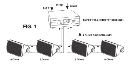
Be sure to use a good quality, unshielded twisted pair speaker cable to connect the amplifier to the speaker(s) (#14AWG for runs <80', #12AWG for runs >80'). Standard ZIP style speaker cable may also be used if twisted pair cable is not available.
