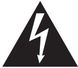
The lightning bolt within arrowhead symbol, within an equilateral triangle, is intended to alert the user to the presence of un-insulated “dangerous voltage” within the product’s enclosure that may be of sufficient magnitude to constitute a risk of electrical shock to person.
