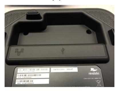
Connect one end of the Ethernet cable into the network connection port on the bottom of the unit. It's characterized by the icon displayed below. Press until it clicks into place.
