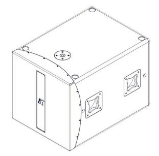
The K-array KMT21 I is a full-featured audio systems featuring a powered 21" subwoofer, programmable onboard DSP and multiple analog and digital inputs and outputs for creating a wide array of speaker configurations. The amplifier mounted on board is class D, delivering 2 x 2400 W at  $4\Omega$ .
