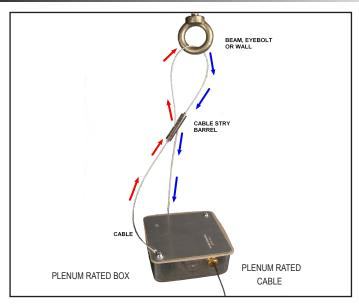
Wrap the cable through fastening point (beam, eyebolt). Next, slip the cable through the top of cable stay barrel pulling excess cable until taut.
