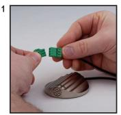
The M60 ships with the male Phoenix connector already attached to the wire, however, a complete set of male and female connectors are provided for your convenience. Disconnect the female Phoenix connector from the assembly by simply pulling apart.
