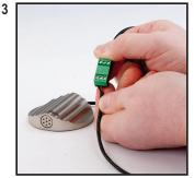
Once wires are firmly attached, reconnect both Phoenix terminals making sure that they are fully engaged and secure.
