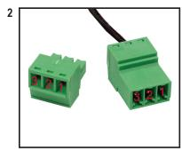
Wiring Scheme: 1 = Ground 2 = Blue (+) 3 = Yellow (-) Strip back wire and attach to the screw on terminals per the wiring scheme. Recommended wire for the M60 is: Belden 9451P with .124" O.D. or Belden 82761 with .116" O.D.
