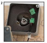
Insert plenum cable through strain relief nut, then connect to the terminal. Recommended cable: Belden 9451P - .124" O.D. or Belden 82761 - .116" O.D.
