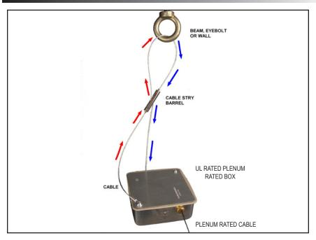
Wrap the cable around a beam, eyebolt or hanger. Next, slip the cable through the top of cable stay barrel pulling → excess cable until taut.
