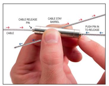
To release cable, depress the cable release pin on either end to release the loop or to extend cable length.
