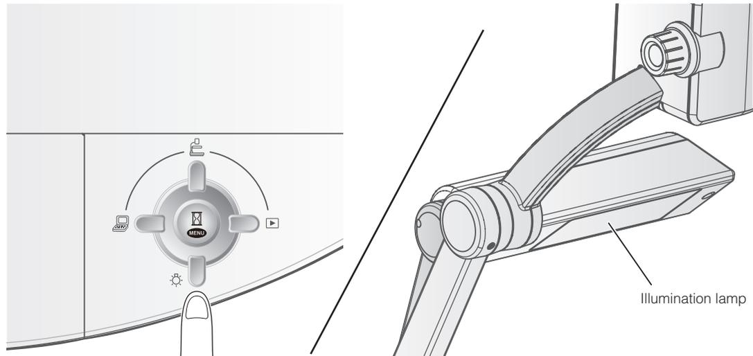
After confirming that no icons are displayed on the screen, press [
