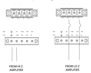
"NOTE: There are four shorting links installed on the 4 position barrier strip. Two are used in each position and are "stacked" in parallel. ALL four shorting links must be removed for Low Z operation. ALL four shorting links (two in each position) MUST be used for Hi Z (70Vrms or 100Vrms) operation." Full wiring instructions for Hi Z and Low Z operation are found on the last page of the product data sheet.
