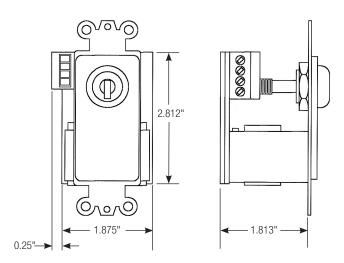
Wiring & Schematics: KL100 Series volume controls (without priority paging feature).
