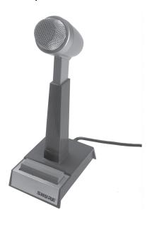
The Model 522 is a dynamic base-station microphone for radio communications, paging, and dispatching systems. Its cardioid (unidirectional) pickup pattern suppresses unwanted background noise from nearby dispatchers, ventilating equipment, or office machines. It also can reduce feedback in public address paging applications.
