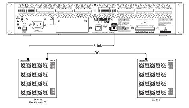
A DX Hub can be connected to the SLink port for further expansion with up to 8 DX expanders. It also enables a single cable link to the AHM-64 processor in cases where multiple expanders are located on a different floor, area or building.
