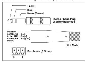
of less than 10 feet are generally ok, but for greater distance or noisy field environments, use balanced input signal wiring.
