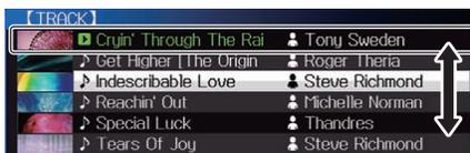
The jump function can be used by pressing the rotary selector for over 1 second.
