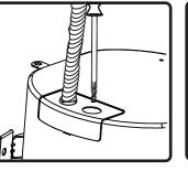
5. Tighten screw on terminal 6. Insert speaker into plate, and push conduit connector into knockout.
