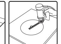
1. Unpack speaker & set 2. Use included tile bridge 3. Use Rotozip or other tool 4. Run signal wires through to cut hole. Hole Diameters CM42-EZs-II 165.1 mm (6.50 in)
