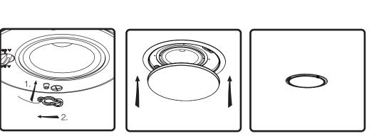
9. Select the tap position by 9. Attach grille safety clip by 10. Press grille into place. 11. Done! adjusting rotary switch to desired high impedance clip over snap-fit post (1), value or voice coil direct mode.
