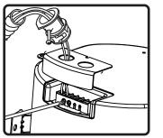
conduit connector, then through cover plate. Connect to ceramic terminal strip. Two + and two connectors are provided for All other CMEZ, FS and BGM models daisy chaining.
