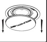
8. Once all painting and finish work is completed, remove the paint mask.
