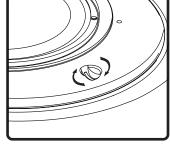
9. Select the tap position 9. Attach grille safety clip by 10. Press grille into place. 11. Done! by adjusting rotary switch placing the large end of the to desired high impedance clip over snap-fit post (1), value or voice coil direct then sliding clip until small mode.
