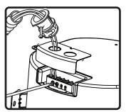
conduit connector, then through cover plate. Connect to ceramic terminal strip. Two + and two connectors are provided for
