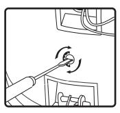
4. Set tap to proper setting. CM-EZ-8 is factory preset in the 70.7 Volt mode in the 20 Watt setting.
