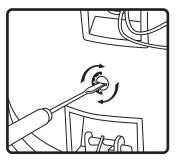
3. Set tap to proper setting. CM-EZ-8 is factory preset in the 70.7 Volt mode in the 20 Watt setting.
