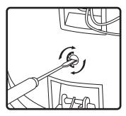
**4.** Set tap to proper setting. CM-EZ-8 is factory preset in the 70.7 Volt mode in the 20 Watt setting.
