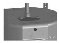
**METHOD 2:** Use any of the three knock-out points at the sides of the backcan (19 mm, 22 mm or 28 mm diameter). (Fig 5)
