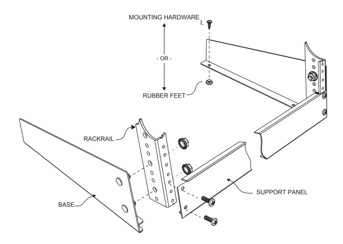
**NOTE:** The mounting hardware can be used in place of rubber feet for additional stability.
