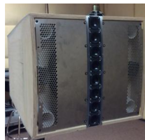
Fig. 7. Oblique view of prototype cabinet with four front-mounted circular ports located in each corner of the front. The cabinet includes a curved-front metal baffle that covers the whole front of the cabinet. The metal baffle is solid for roughly 127 mm (5”) on either side of the HF array and perforated the rest of the way so that the acoustic output of the LF driver and ports can escape to the outside.
