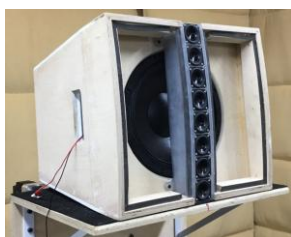
Fig. 6. Oblique view of prototype cabinet before ports were added on the front.
