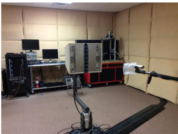
Fig. 11. Measurement setup for gathering on- and off-axis frequency response measurements. The Four Audio ELF automated loudspeaker measurement system was used for these measurements. Rotation was about the cabinet front with the test microphone 2 m from the front of the box.
