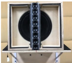
Fig. 5. Front view of prototype cabinet constructed of 19 mm Baltic Birch plywood. This photo was taken before the ports were added to the front of the enclosure.
