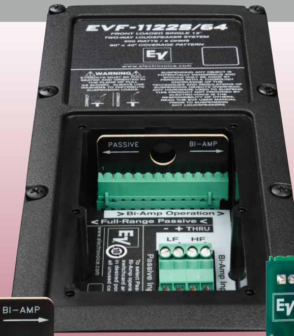
The plug-in card system is a unique feature of the EV-Innovation family of loudspeakers. This simple device (EVI-AC) allows diagnostic access to the transducers and protection circuitry inside the enclosure WITHOUT requiring any disassembly or disconnections beyond simple removal and replacement of the plug-in passive/biamp switch card. The EVI-AC works with all EVA, EVF and EVH two-way and low-frequency systems with plug-in card.
