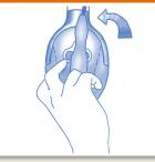
Microphone mutes automatically when boom is set to "UP" position.
