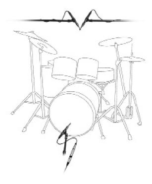
Figure 4. Overhead miking with VERTICAL X/Y positioning
