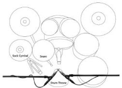
Figure 1. Overhead miking with HORIZONTAL X/Y positioning
