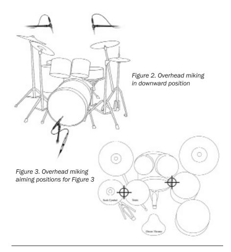
All of the microphone positionings shown in Figures 1-4 should provide excellent results using an Earthworks DK25 Series DrumKit three microphone system.
