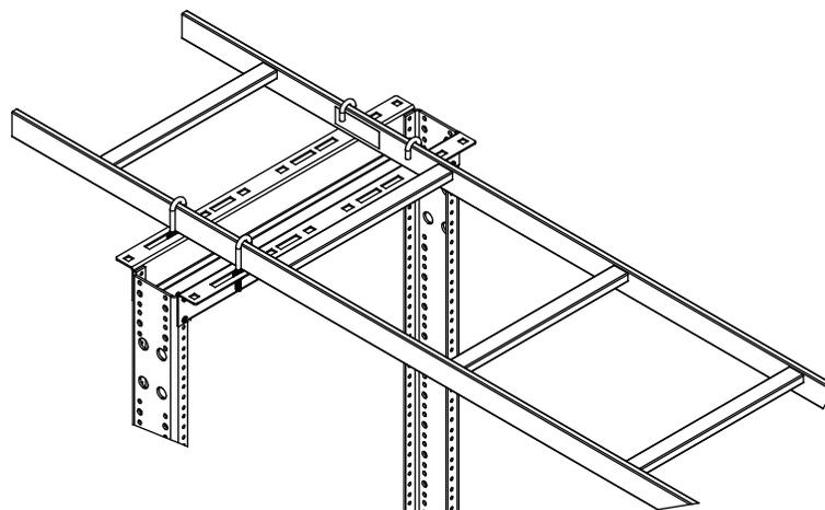
**Optional Cantilever Support Base allows cantilevered equipment to be safely installed in the RL Series.**
