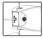
8. Select desired location for safety cable and remove the U-bracket screw from that side. Attach safety cable to the clamping screw and reinstall loosely.
