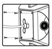
7. Install back plate and secure with included fasteners.
