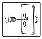
4. If being installed per EN54-24 regulations or in instances where a water tight strain relief bushing is necessary, attach the included strain relief bushing to the back plate. If it is not required, skip this step.
