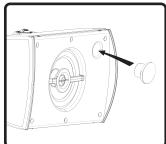
To enhance protection of internal components from humidity and other potentially corrosive elements, use provided port plug to seal enclosure. Use RTV silicone around edge of the port plug for increased protection. Note: WX versions will come with the port plug pre-installed.
