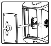
5. Run signal wires through cstrain relief bushing then connect to ceramic terminal strip. Two + (plus) and two -(negative) connectors are provided for daisy chaining.
