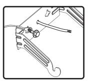
clamping slots pointing upward. Securely fasten mounting bracket and safety cable to surface (user must supply fasteners). Note: The safety cable will
