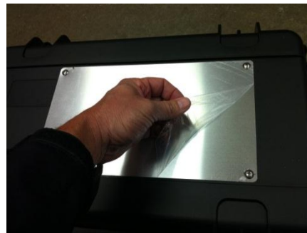
Remove protective plastic covering from face of plate
