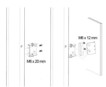
$\label{thm:condition} \textbf{See COL Column Speaker Installation Guide for further information and details about installing this loudspeaker.}$
