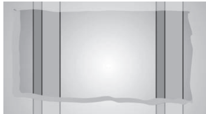
Figure 1 Cut an opening large enough to install the mounting bracket to the wall studs
