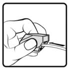
**2**. Thread hanging cable through Gripple as shown
