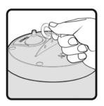
5. The hanging cable should be attached to the centre hole on the bracket.
