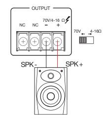
**70 Volt speaker:** According to the rated power of the power amplifier, adjust the 70V transformer tap accordingly.
