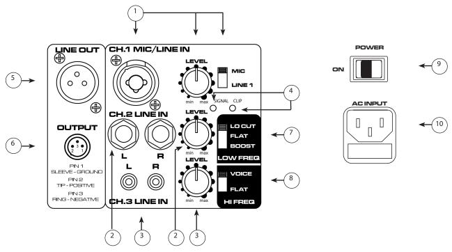
1) **CHANNEL 1 INPUT**: XLR combi 1/4" input with mic/line pad switch.
