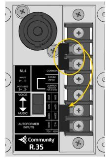
Must remove jumper, or move it to the bottom terminals, for  $8\Omega$  operation (see yellow arrow)
