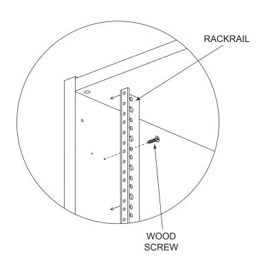
**NOTE:** When moving front rackrail to setback position, mount rail to recessed pilot holes on opposite end of side panel. This hides the original mounting holes from view.
