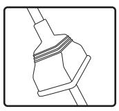
2. Slip terminal weather boot over signal wire. For environmental applications, put RTV silicone around nipple and base when installation is complete.
