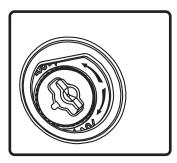
1. Select the tap position by removing the rubber plug on grille to access rotary switch. The tap switch has 2 settings: 4 ohm and 36 ohm (for 70.7V 138W/100V 276W). Select the desired setting and reinsert rubber plug. **Note:** The grille-mounted tap switch cover is keyed; be sure flat edge of plug lines up with flat edge of hole in grille.
