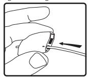
**5.** Thread hanging or safety cable through SpeedClamp<sup>™</sup> mechanisms as shown
