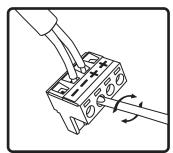
**3.** Connect signal wire to 4-pin Euroblock plug. Tighten unused terminal screws. Use inside positive and negative inputs for either voice coil or distributed systems. For daisy chaining, use outside positive and negative terminals.
