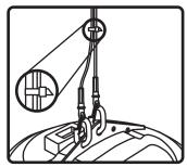
**12.** Use zip or twist-lock ties to secure safety cable & signal wire to main hanging cables. Cable cover available for asthetic applications (SLT-10).
