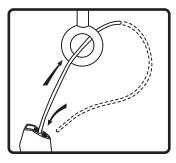
**6.** Attach the hanging cable by securing it and safety cable to structure as shown.
