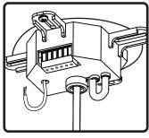
5. Connect Signal wire into terminal block
