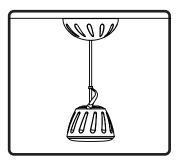
10. Completely thread cover plate to secure speaker.
