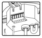
6. RS31-EZ-T wiring: Connect the negative signal wire to "com" and the positive signal wire to the desired power tap as indicated.
