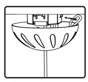
9. Excess wire can be hidden inside of cover plate by wrapping excess wire clockwise and into gap between plate and surface
