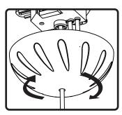
8. Move cover plate up speaker wire, begin to thread cover plate into mounting plate, leaving half an inch between cover plate and mounting surface.
