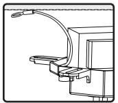
3. Where needed, connect safety leash to secure point on structure/junction box.
