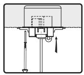
4. Screw mounting plate into the junction box (not included) using the moutning screws provided.
