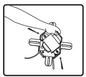
2. Remove the input module mounted onto the transformer. Unscrew to remove the transormer.
