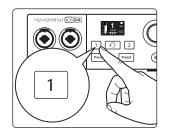
To set your Revelator io 24's input level, press the Channel button for the Channel you would like to use. Next, press the encoder to cycle through the available options. A yellow underline will indicate the currently-selected option. Once you've selected the Gain setting—it's shown below the Channel indicator number and measured in dB (decibels)—turn the Encoder to set the desired gain level.
