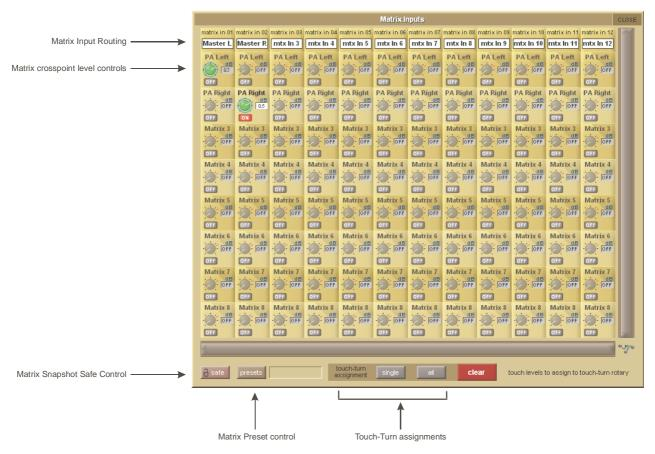
The example above has the Master Stereo Buss routed to the inputs of Matrix 1 and Matrix 2 (Labelled as PA LEFT & PA RIGHT). By adjusting the crosspoint levels, you can change how much of each side of the Master buss is fed to these Matrix Channels.
