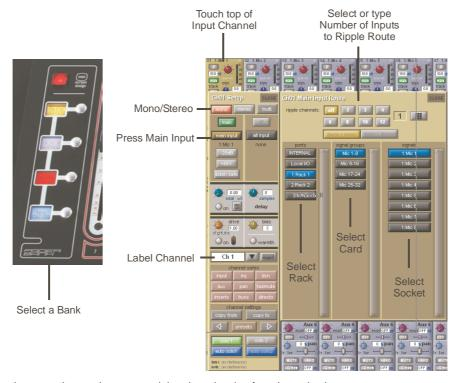
Within each display, there are three columns containing three levels of routing selection:
