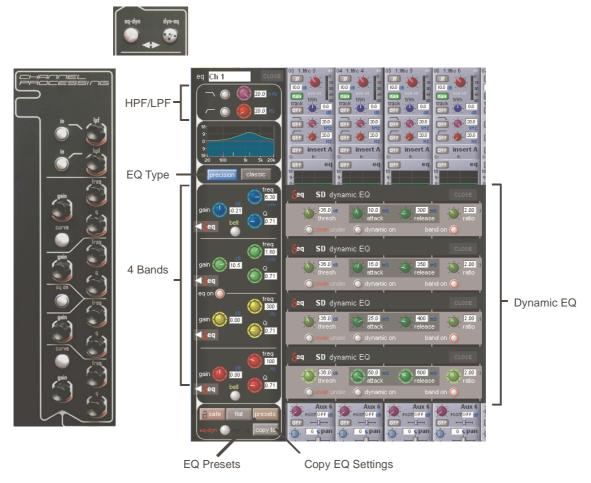
The type of filter used by the top and bottom bands can be changed by successive presses of the **Curve** button for that band. The four parametric bands can be either **Classic (Analogue style)** or **Precision (Digital style)** type EQ.
