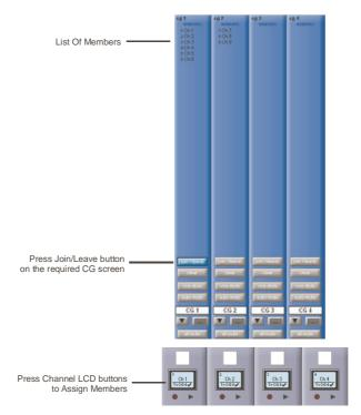
A list of all the connected channels and their names is displayed above each Control Group display. You can also clear all the channels from a Control Group by pressing **Clear**.
