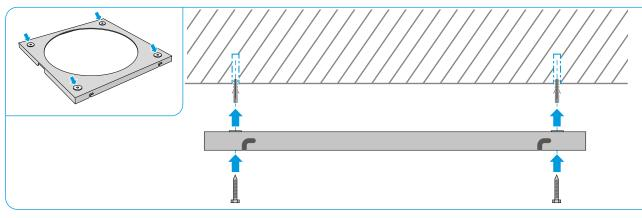
> Attach the ceiling fixation bracket to the ceiling using adequate screws and anchors.
