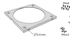
Screws and anchors for attaching the ceiling fixation bracket to the ceiling are not included. Make sure to use adequate screws and anchors for the installation, depending on the material characteristics of the ceiling.
