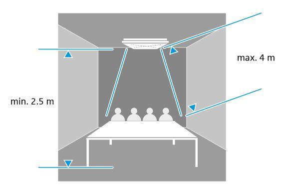
The recommended distance between the person speaking and the SL Ceiling Mic should not exceed 4 m.
