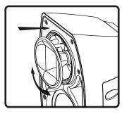
3. To replace horn assembly, insert horn 1/8 turn from final position and rotate clockwise to tighten. Horn is fully engaged when horn baffle throat is aligned with speaker.
