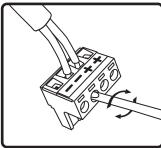
5. Connect signal wire to four-pin Euroblock plug. Use inside positive and negative inputs for either voice coil or distributed systems. For daisy chaining, use outside positive and negative terminals. Tighten unused terminal screws.
