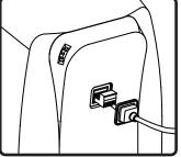
6. Insert four-pin Euroblock jack on rear of speaker. Connectors are keyed for polarity.
