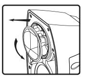
2. To release the horn, insert hand into horn throat and twist horn assembly counter-clockwise.
