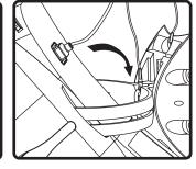
8. Clip snap link with safety cable to mounting bracket.
