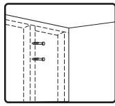
2. Choose a secure mounting surface with sufficient strength to reliably hold the speaker. Mounting bracket accommodates screwing, throughbolting and strapping installation options. The max. strap width is 0.73 in / 18.5 mm.
