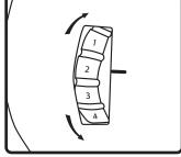
9. Select the desired setting on the rear-mounted tap switch. Use table to right to choose appropriate tap number based on system voltage, and desired power draw.
