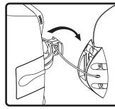
7. Slide speaker into wall mount plate until it locks into place.
