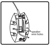
3. Feed speaker wire through speaker wire hole before mounting. Thread safety cable (included) through mounting screw and securely fasten mounting plate to surface (user must supply fasteners). Mounting bracket may also be strap-mounted to pole or appropriate anchor point.
