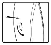
4. Attach grille by pressing down gently and rotating the retention knob clockwise to vertical postion.
