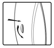
1. To rotate the horn, disengage grille by rotating the retention knob counter-clockwise to horizontal position while gently pushing down on the grille.
