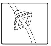
4. Slip terminal weather boot over signal wire. For environmental applications, put sealant around nipple and base when installation is complete.
