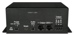
The Contemporary Research SMG-40 Sound Masking Generator has the power to drive over 30 25V plenum and ceiling speakers, 70V transformer, 4/8 ohm speakers, and over 100 Cambridge Qt® Emitters. Many masking generators use standard pink noise while the SMG-40 filtered noise is optimized for masking speech in real-world applications.
