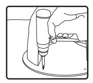
7. Set speaker enclosure on speaker base. Use tamperresistant stainless-steel screws to attach speaker to base (driver tip and screws provided).
