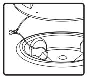
6. Attach signal wire to wire leads. Use wire nuts provided. For added water proofing, grease caps are recommended.
