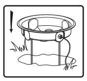
4. Place speaker base into hole in ground with the top rim of the base at ground level. Back-fill dirt in to hole, packing the dirt firmly. For added security, cement security brackets into ground.
