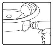
1. If needed for daisy chaining drill speaker base and install second liquid-tight strain relief (not included).
