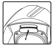
To enhance bass performance, remove port cover on the underside of speaker enclosure. Warning: Removing the cover will expose internal components to humidity and other potentially corrosive elements.
