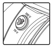
5. Select the tap position by removing the rubber plug to access rotary switch. Switch is preset to maximum tap setting in 70.7 V mode (64W XT850, 32W XT550). Select desired setting and reinsert rubber plug.
