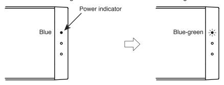
**Step 2.** Hold down the Power switch while confirming that the Power indicator is flashing blue-green.
