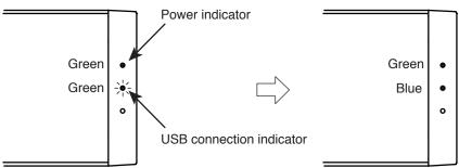
**Step 3.** After ensuring that the USB connection indicator is lit blue, release the Power switch.
