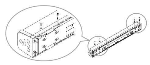
**Step 2.** Attach the wall mounting bracket to a wall.
