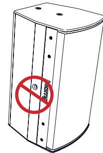
The loudspeaker enclosure must have fasteners in all threaded holes
