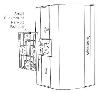
Pivot angle (portrait orientation) Horizontal 120° in 10° increments Vertical 56° in 8° increments
