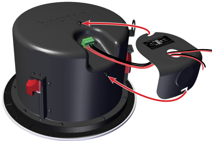
Figure 6. Wire loudspeaker (conduit not shown)
